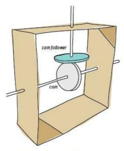
The spinning element that you turn with the handle is called a cam. The element that sits on top of the cam will move according to the shape and position of the cam, and is called a cam follower. The cam follower transmits its motion to the elements on top of the box to animate your sculpture.
